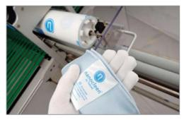
World leading Teknek Nanocleen<sup>™</sup> cleaning core. Nanocleen<sup>™</sup> is a silicone and static free system that is capable of cleaning particles smaller than 1 micron. Ideal for thin, sensitive materials such as polyimide, polyester, copper etc.
